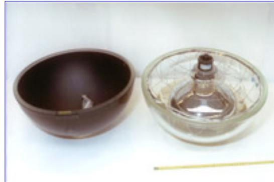
The Optical Module (OM) is a glass sphere containing a photomultiplier (PMT), the light-sensitive element of the ANTARES detector. The glass sphere consists of two hemispherical parts. One hemisphere holds the PMT. The other hemisphere is equipped with an electrical penetrator, a vacuum port and a manometer, and is covered, inside, with black paint.
