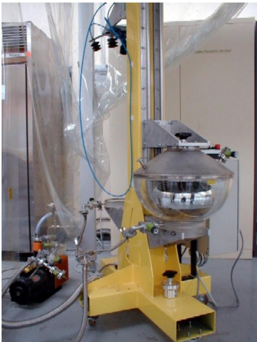
In this picture, the photomultiplier and the cage are glued in the hemisphere, waiting for polymerisation of the gel.
