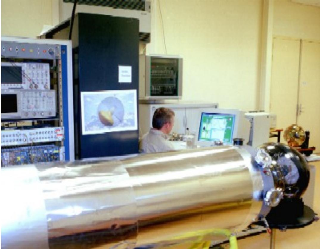
The cylinder in the foreground is the "black box" in which the photomultiplier is tested. It is surrounded by a  $\mu$ -metal sheet. On the right, one can see an Optical Module ready to be introduced in the cylinder. A blue light source is situated at the other end of the cylinder.
