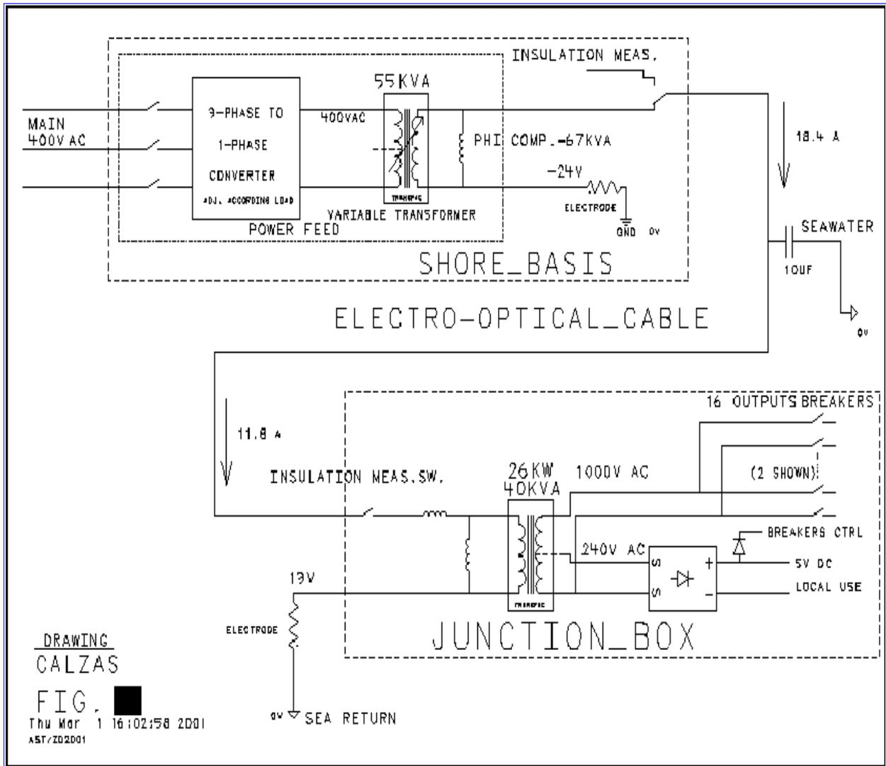
**Figure 7.1** Schematic diagramme of the Electrical Power system
