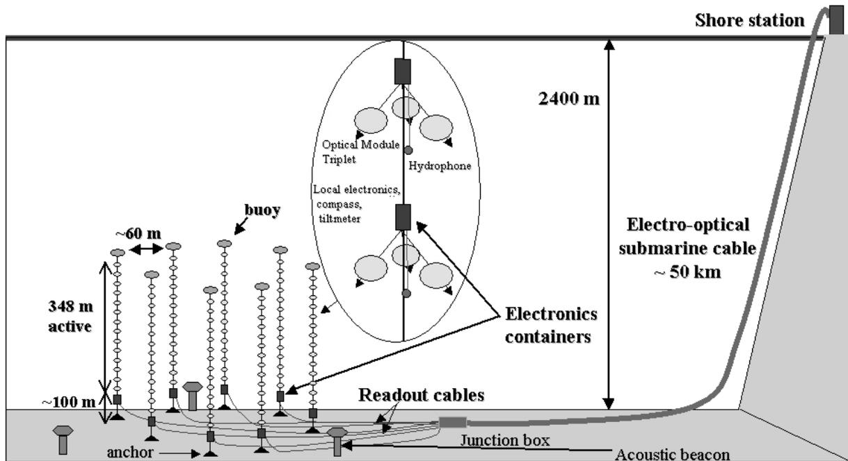
Fig. 1. Schematic view of a part of the detector (the full configuration will consist of 10 strings). The magnified view encompasses two storeys.
