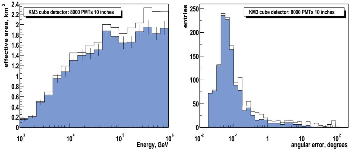
Figure 1: Results of the Monte-Carlo simulation of the km<sup>3</sup> detector: Effective area of the detector as a function of muon energy (left plot). Angular error in muon track reconstruction (right plot). The results with the quality cut are shown on the figure as shaded area. Error bars on the left plot show statistical errors only.
