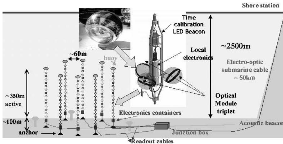
Figure 1: Schematic view of the ANTARES detector.
