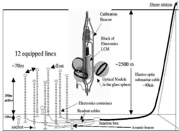
Fig. 1. Schematic view of the ANTARES detector
