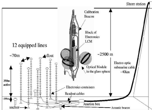
Figure 1. Schematic view of the Antares detector.
