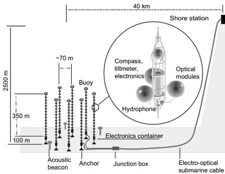
Figure 1: Schematic view of the ANTARES detector
