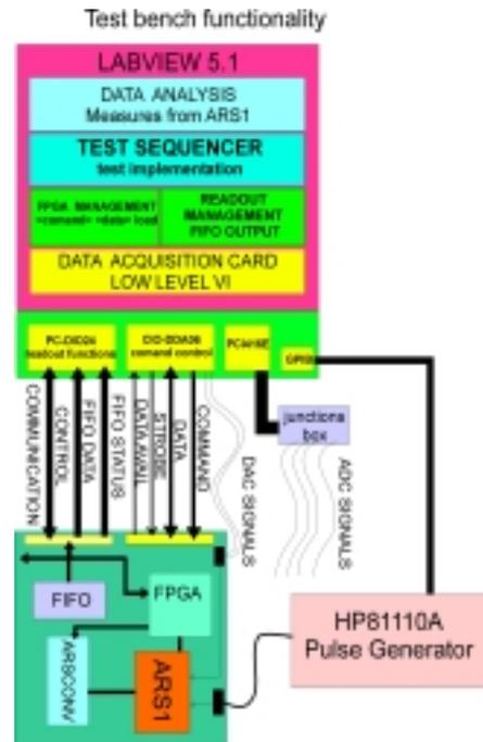
Figure 3: Test bench architecture.
