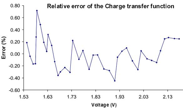
Figure 11: Example of Integral linearity error of one ARS1
