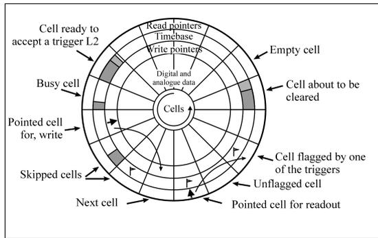
Figure 13: Examples of the pipeline management.
