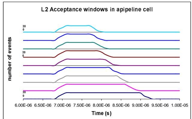
Figure 14: Example of acceptance window measurement.
