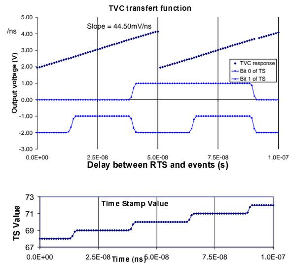
Figure 12: arrival time transfer function of an ARS1.
