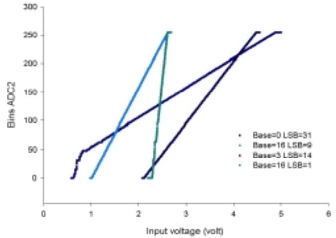
Figure 16: transfer function of 8 bits ADC for four bank of values
