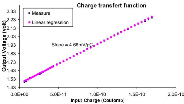
Figure 10: Examples of Charge transfer function
