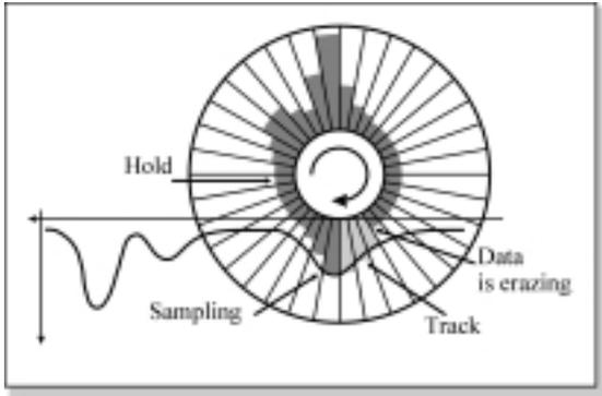
Figure 5: Ring Sampling principle
