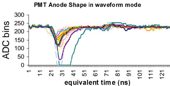
Figure 7a: Examples of anode shape
