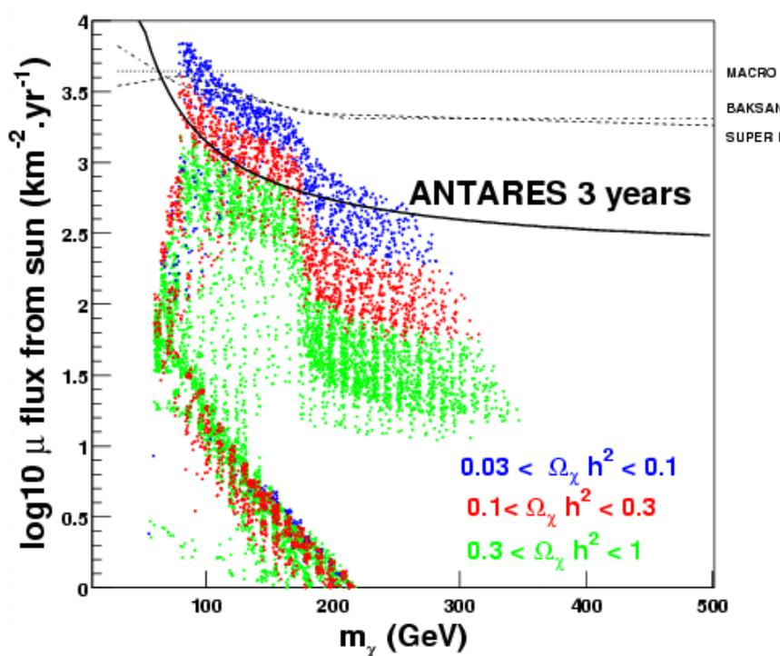
Fig. 1. ANTARES sensitivity to a muon flux from neutralinos in the Sun.
