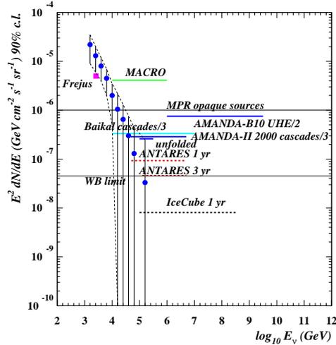
Figure 6. ANTARES sensitivity to diffuse fluxes as a function of the neutrino energy. The upper limit that can be set by ANTARES after one year and three years of data taking are shown together with theoretical predictions and results of other experiments. The circles show the atmospheric neutrino spectrum measured by AMANDA (see [8] for references of the theoretical models and experimental limits).
