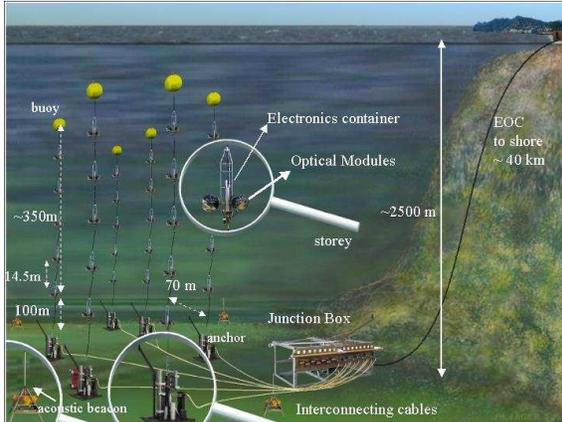
Figure 1. Schematic view of the ANTARES detector.
