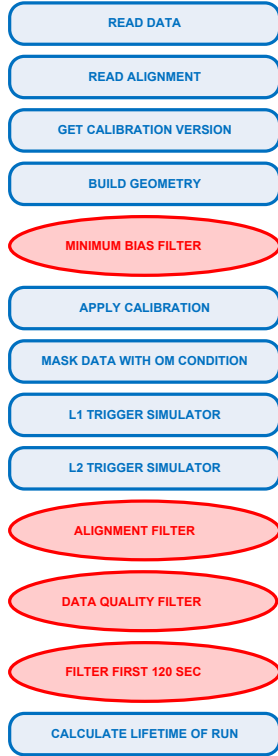
Figure 5.1: Scheme of the data processing chain of the present thesis. The data has been processed within the SeaTray software framework.
