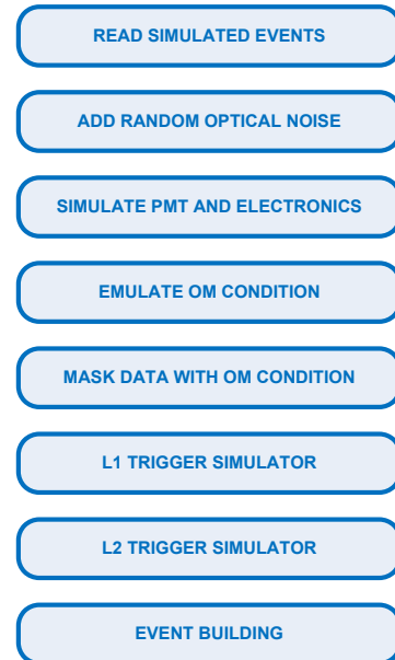
Figure 5.2: Scheme of the simulation processing chain of the present thesis. The simulations have been processed within the SeaTray software framework.
