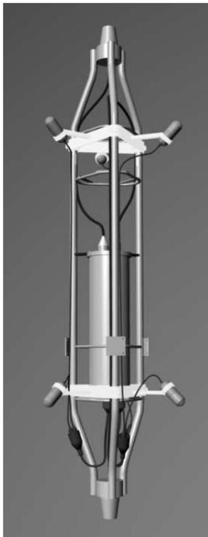
Figure E.1: *Illustration of an acoustic storey. The three optical modules, which are part of a standard storey, have been replaced by six hydrophones. The image has been taken from [61].*
