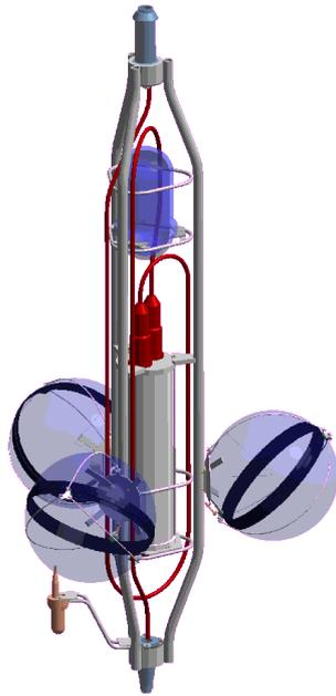
Figure 4.4: Drawing of an ANTARES storey. The three Optical Modules, the electronics cylinder (grey), the LED-beacon (blue) and the hydrophone (ochre) for acoustic positioning are visible (figure from ANTARES internal pages).
