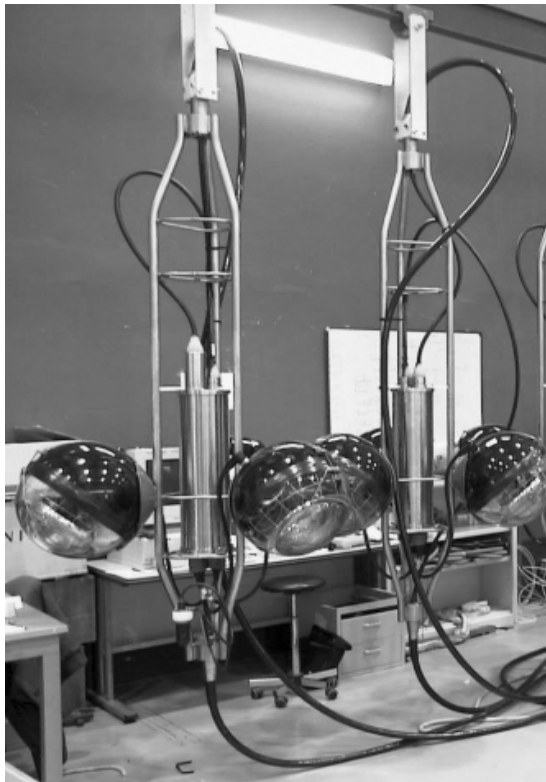
Figure 1.3: Photograph of two fully integrated storeys. A titanium frame supports three optical modules that are connected to the local control module which contains the control and read-out electronics. The frame also provides the mechanical connection to the electro-mechanical cable that interconnects the storeys.
