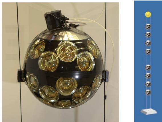
Figure 2.6: On the left, a KM3NeT DOM. On the right, a simplified view of a KM3NeT DU (note that only part of the DOMs are shown, for better visibility of the scheme).
