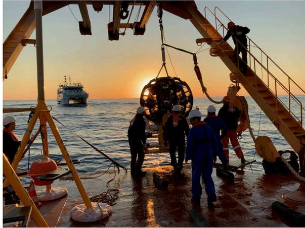
Figure 2.8: A picture of a DU deployment, where the detection unit is furled into the LOM.
