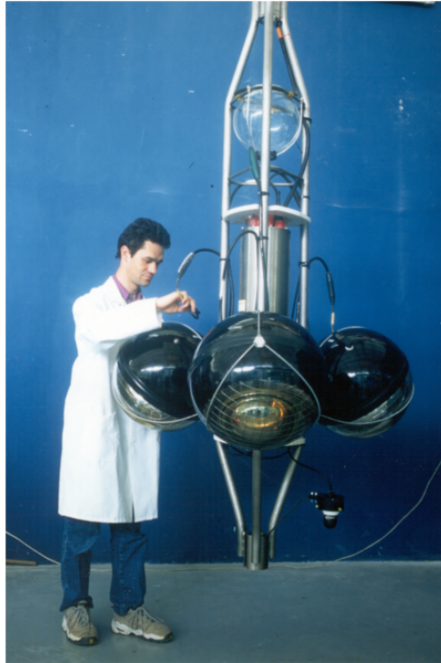
Figure 10.1: An ANTARES storey with three OMs. Taken from [170].
