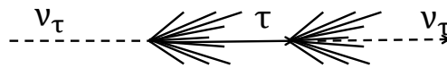
(b) CC interaction of a \nu_\tau producing an hadronic shower and a charged tau lepton that decays into another \nu_\tau after some distance, generating another hadronic shower
