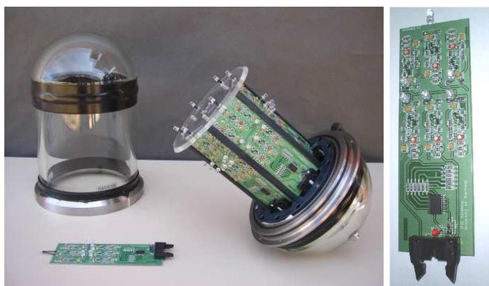
**Figure 3.8:** Left: one of the LED Beacons used for the ANTARES time calibration. The picture shows the hexagonal frame with the 36 LEDs, and the glass container designed to protect the device once has been deployed. Right: a face of the LED Beacon.
