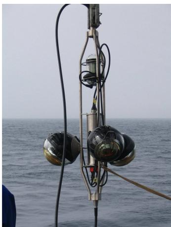
**Figure 2.8:** Picture of a storey being deployed. There are 3 OMs facing  $45^\circ$  downward, and the LCM in the center housing the readout electronic cards. An LED Optical Beacon for timing calibration purposes can also be seen in the top part of the storey frame.
