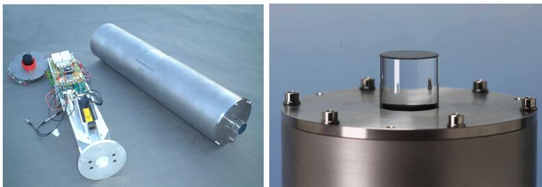
**Figure 3.12:** Left: one of the Laser OBs used for the ANTARES time calibration, showing the titanium frame, the laser and its electronics. Right: the quartz rod through whose vertical walls spread the laser light to all the detector.
