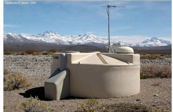
Figure 3.3 – Water Cherenkov station. It contains 12 000 liters of pure water and three photomultiplier tubes.
