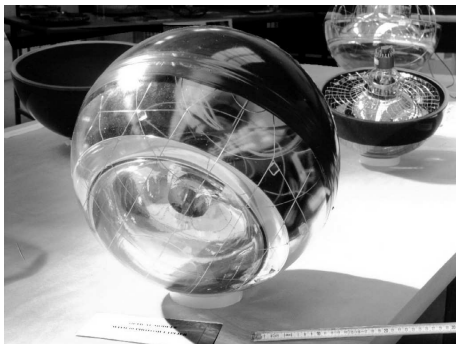
Figure 2.2: A photograph of an Optical Module. The 10" photomultiplier tube, the \mu -metal shield and the black paint can be seen inside the glass sphere. The electronics and the connection point are not visible in this photograph.
