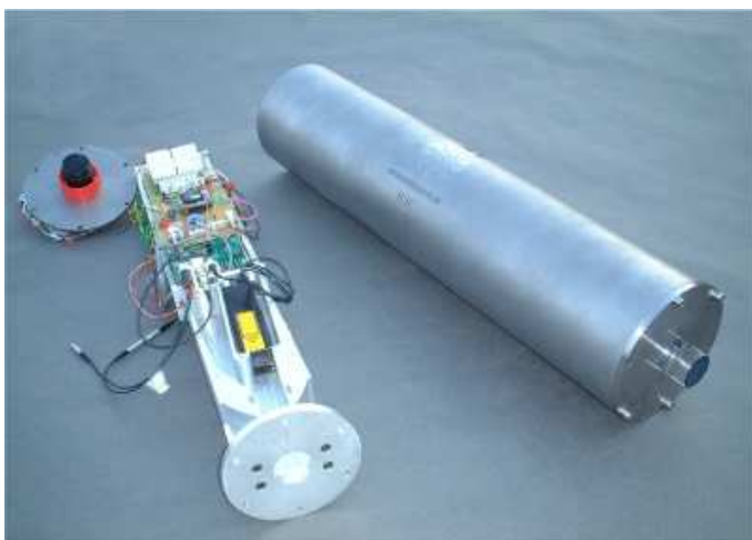
Figure 3.2: A Laser Beacon dismantled: On the left of the picture, the inner mechanics holding the laser head and its associated electronics. On the right, the pressure-resistant titanium container that houses the equipment. On the top end plate of the container (right part of the picture) the quartz cylinder that prevents sedimentation effects.
