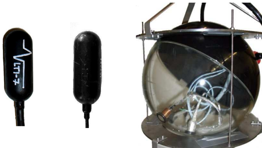
Figure 6.2: Photographs of the sensors used in AMADEUS. From left to right: Custom-designed hydrophone, commercial hydrophone and Acoustic Module (AM). The AM is a prototype with three active elements mounted in a mechanical structure for calibration measurements.
