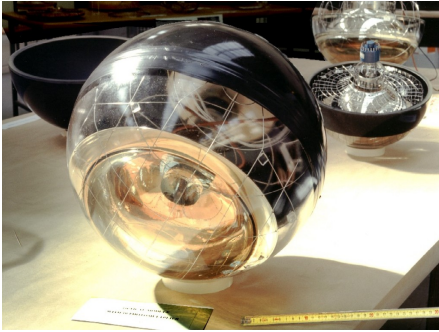
Figure 5.2: Optical Module of the ANTARES detector [27].
