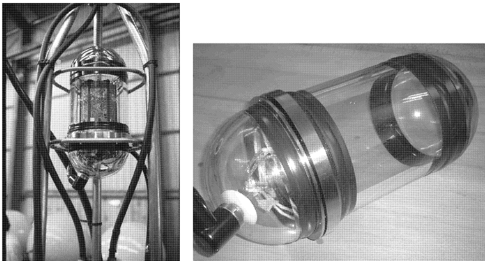
Figure 3.8: The Optical Module Frame with one LED Beacon (left side). The LED Beacon borosilicate glass container (right side).
