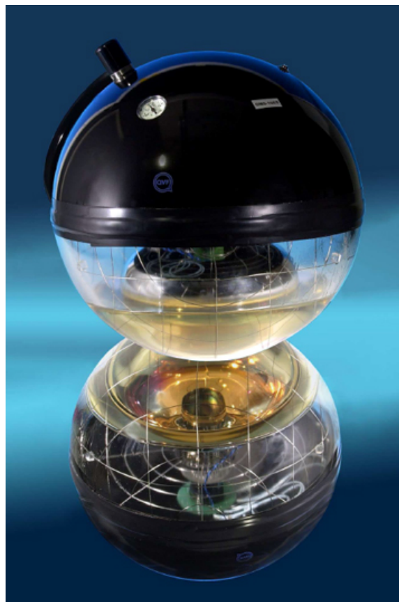
FIGURE 1.9: A picture of an Optical Module showing also its components.
