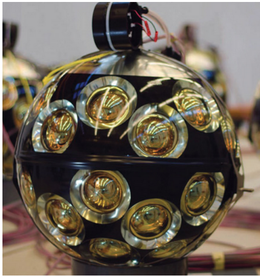
FIGURE C.2: Photograph of the digital optical module.
