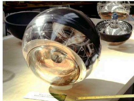
Figure 2.9: Schematic view of an Optical Module showing its different components (left). Picture from an OM at the integration site (right).
